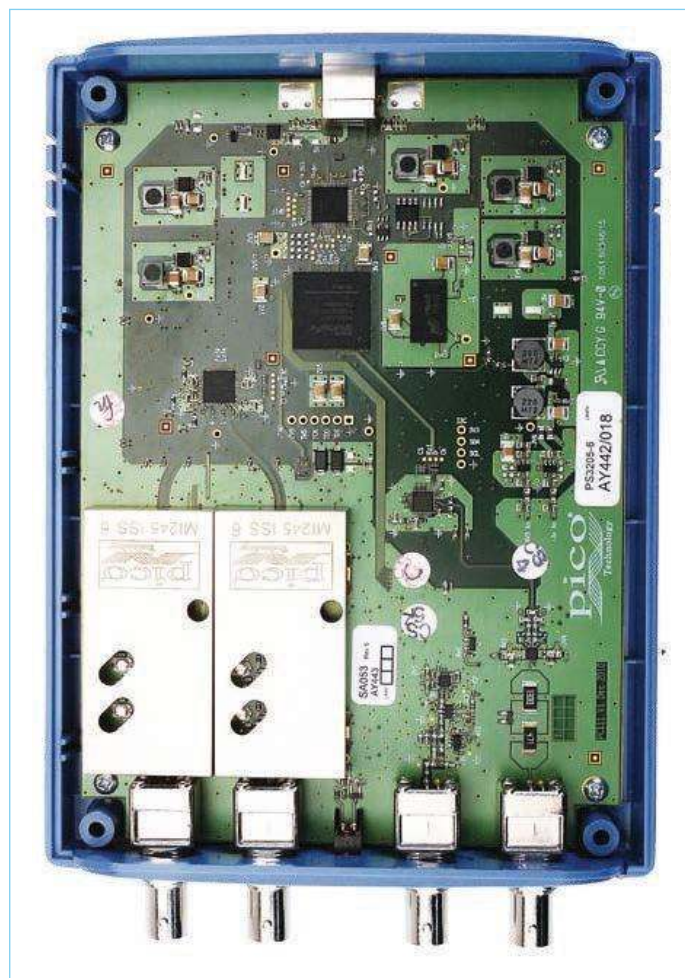
Figure 1. The inner workings of the new 3000 series from Pico. Note the shielded input sections.
