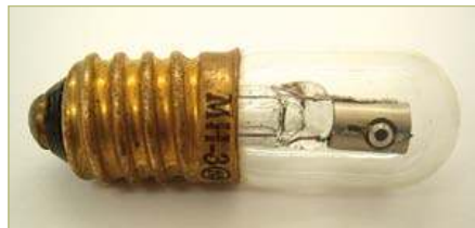
Figure 9. A gas discharge tube with a radioactive ioniser to aid starting.
